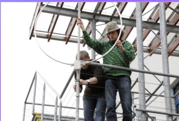
Installation of SID monitor antenna – detector of radio VLF disturbances as alternative method to detect gamma-ray bursts
