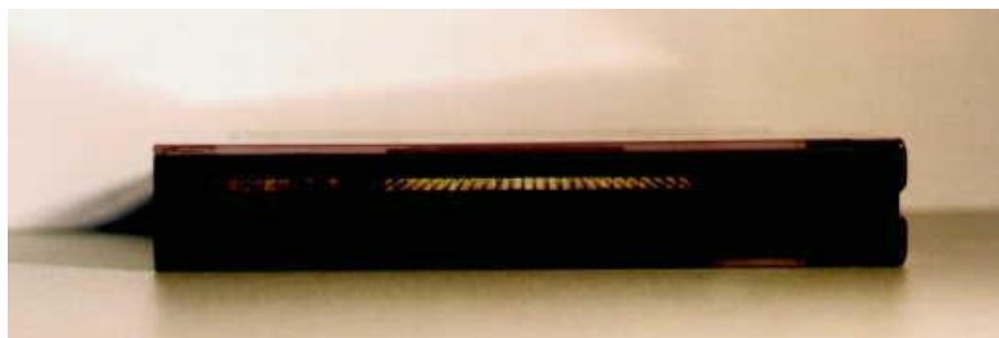
Angel telescope linear test module, 47 square cells 2.5 x 2.5 x 120 mm each.
