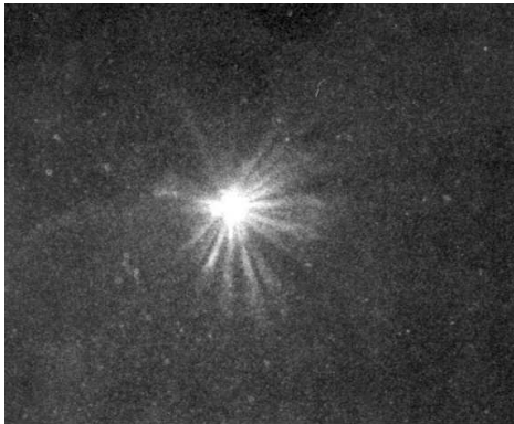
X - ray images of the laser plasma by the 17 mm EH microscope (IPPLM Warsaw)
