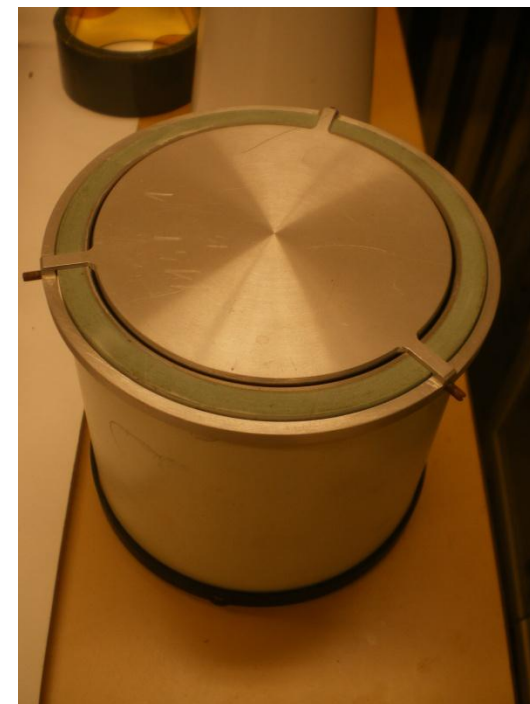
115 mm Wolter, Ni/epoxy, 1979
