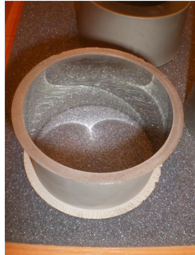
Ultra-thin Ni test mirror (thickness 0.2 mm) 1983
