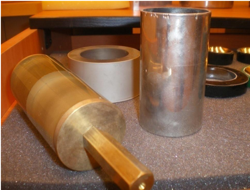
Mandrel (left) and replica (right) Mostly glass and glass ceramics was used for mandrels, 1971
