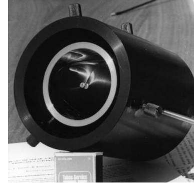
One of the first Czech X-ray Wolter mirrors, 1970, aperture 50 mm
