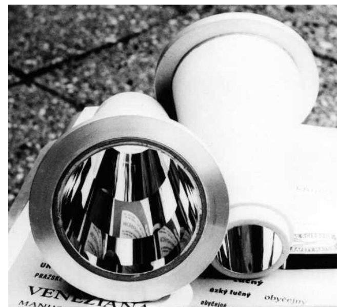
Two identical mirrors (large hyperbolas) of the RT-4M mirror array (Ni surfaces), 1981.
